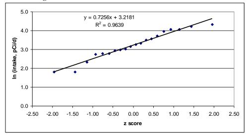
Production workers are assumed to have been continually exposed at the 95th percentile intake rate of 82 pCi/day, and administrative personnel are assumed to be exposed continually at the median intake rate of 25 pCi/day. The total uranium intakes are applied as 50% U-238 and 50% U-234, which allow for intakes of U-235. Intakes of long-lived radionuclides that are significant for internal dose are listed in Table 4a. These bounding intakes should be entered into IREP as constants.
