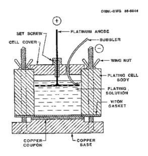
Figure 2: Detailed Drawing of ORNL Plating Cell
