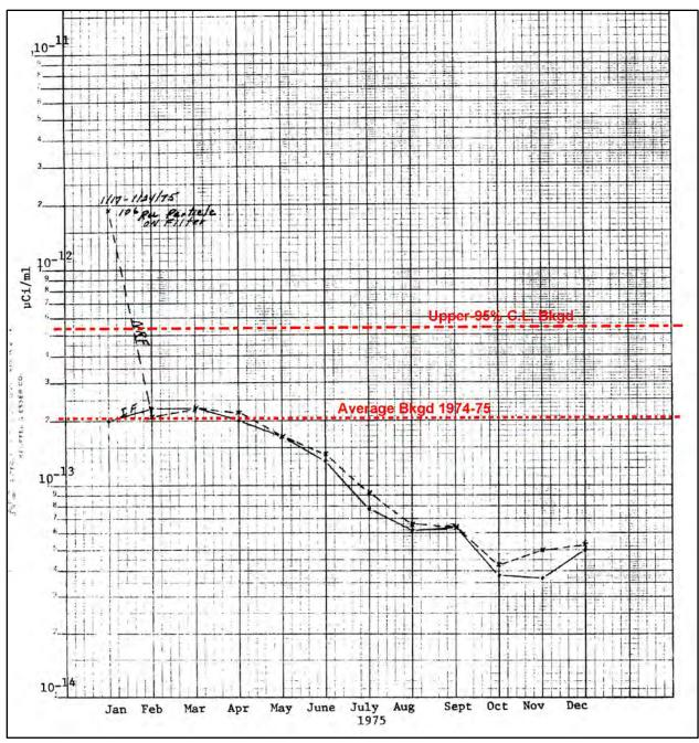
Figure 12 – CY-1975 - Monthly Gross Beta Environmental Air Concentrations at NRF and Background Location at Idaho Falls (Sill 1976)
