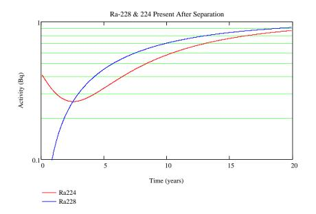
Figure 6. Ra-224 and Ra-228 activity after a second chemical purification which occurred when Th-228 was at its lowest equilibration point (4.55 years) after the first purification.
