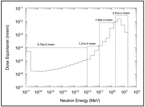
Figure 6.3.4.2-3. Results of PNL neutron spectrum measurements made at 1 meter from a bare <sup>252</sup>Cf fission neutron source are shown by the solid line in the graph and the dash line shows the PNL measurement results divided into the four neutron energy groups used in the dose reconstruction for Y-12 workers at the Nondestructive Analysis Laboratory in Building 9720-5.
