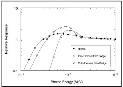
Figure 6.3.2.1-1. Comparison of Hp(10) from a broad beam of normally incident photons (ICRP 1996) with the energy responses for a sensitive DuPont 502 emulsion in a MED two-element film badge (Pardue, Goldstein, and Wollan 1944) and a sensitive DuPont 555 emulsion in an ORNL
