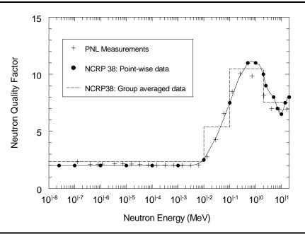
Figure 6.4.2.1-1. Comparison of the neutron quality factors used in the PNL neutron spectrum measurements and the neutron quality factors from NCRP Report 38 (NCRP 1971) shown both as point-wise data and grouped averaged data over the four neutron energy groups used in the dose reconstruction for the Y-12 workers.
