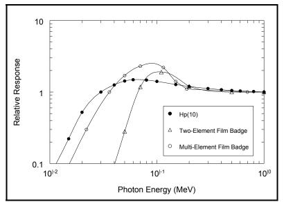
Figure 6.3.2.1-1. Comparison of Hp(10) from a broad beam of normally incident photons (ICRP 1996) with the energy responses for a sensitive DuPont 502 emulsion in a MED two-element film badge (Pardue, Goldstein, and Wollan 1944) and a sensitive DuPont 555 emulsion in an ORNL multi-element film badge (Thornton, Davis, and Gupton 1961).
