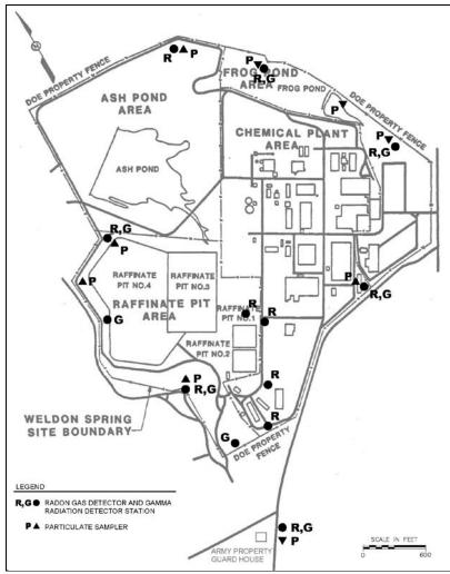
Figure 4-3. Air particulate (P), radon (R), and gamma (G) monitoring stations in WSCP and WSRP.
