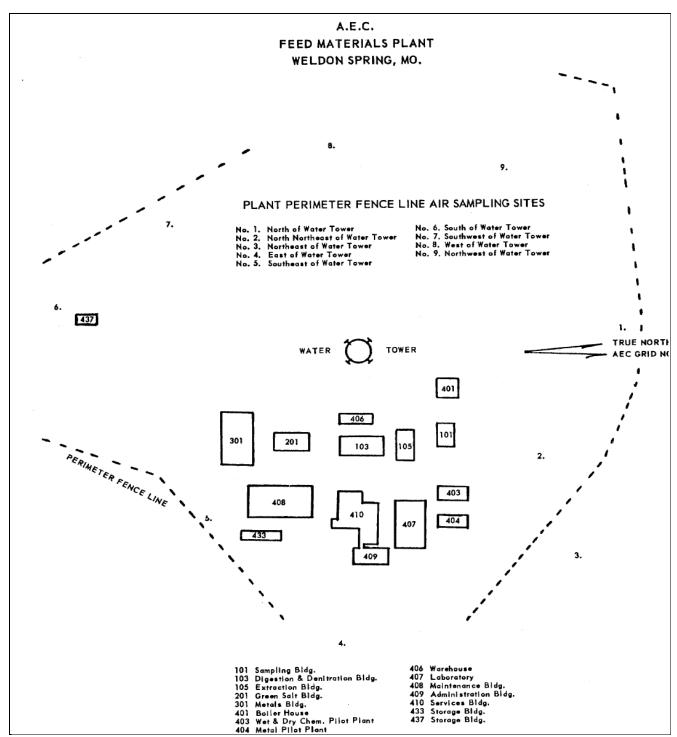
Figure 4-1. Map showing perimeter sampling locations and processing facilities (lacking distance scale).
