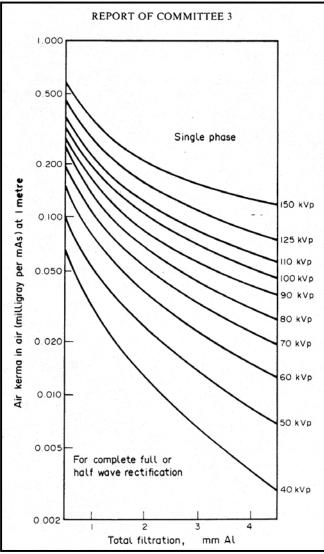
Figure 3-1. Kerma in air at 1 meter from X-ray source as a function of total filtration for various values of tube potential (from ICRP 1982).
