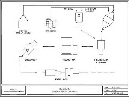
Figure 2-7. UF<sub>6</sub> conversion to uranium metal (adapted from US Army 1976).
