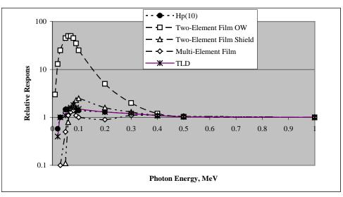
Figure 5.3.2.1-1 Estimated SRS Dosimeter Photon Response Characteristics
