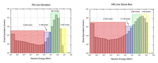
Figure 5.3.4.2-1 Neutron Energy Spectra Recorded at SRS Plutonium Facilities with Neutron Energy Groups Overlay.
