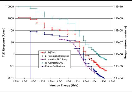
Figure A-6. TLD response for monoenergetic neutrons.
