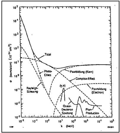
Figure 2-2. Photon cross sections for copper.
