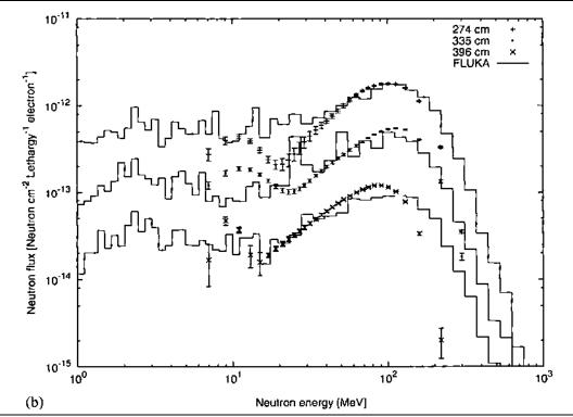
Figure 2-4. Time-of-flight measured neutron spectra through iron and concrete (Taniguchi et al. 2003).
