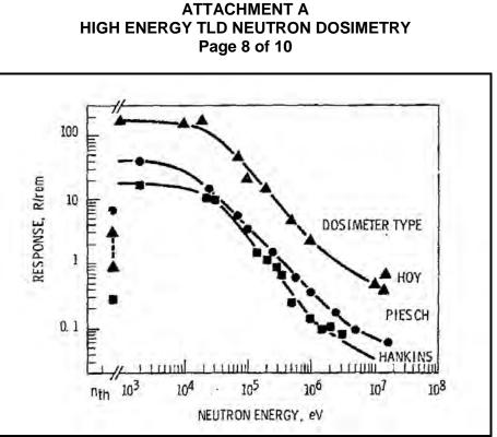
Figure A-5. Energy response of various albedo dosimeters.
