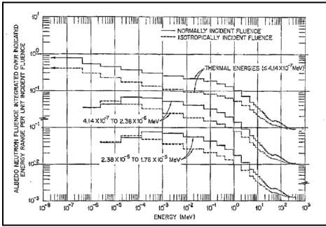
Figure A-4. Albedo-neutron fluence integrated over the specified energy ranges vs. incident neutron energy for monoenergetic neutron fluences normally and isotropically incident on a 30-cm-thick semiinfinite tissue slab
