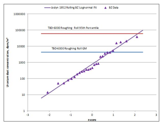
Figure 7-2: Comparison of the Lognormal Fit of the Joslyn 1952 BZ Air Concentration Data to the GM and 95<sup>th</sup> Percentile for the 1951-1955 Roughing Roll Operator Distribution in Battelle-TBD-6000
