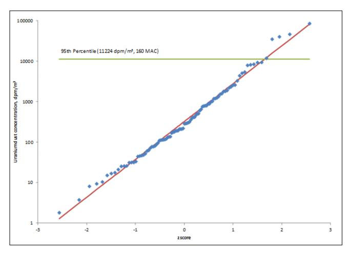
Figure 6-1: Lognormal Fit of All 1952 Un-weighted Air Concentration Data (GM = 323 dpm/m3, GSD = 8.63)
