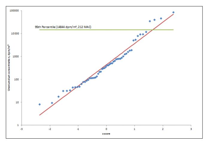
Figure 6-2: Lognormal Fit of the 1952 Un-weighted Breathing Zone Air Concentration Data (GM = 437 dpm/m3, GSD = 8.51)
