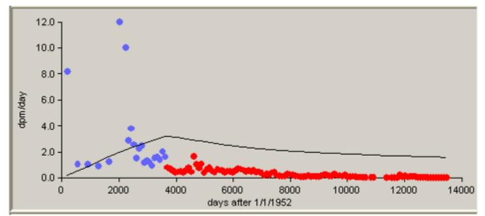
Figure D-36. Predicted plutonium bioassay results (line) calculated using IMBA-derived plutonium intake rates compared with measured plutonium-in-urine results (dots), 1/1/1952 to 12/31/1961, 84th-percentile, Type S.
