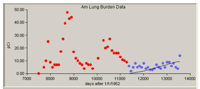
Figure D-45. Predicted americium bioassay results (line) calculated using IMBA-derived americium intake rates compared with measured americium lung burden results (dots), 1/1/1983 to 12/31/1988, 50th-percentile, Type S.
