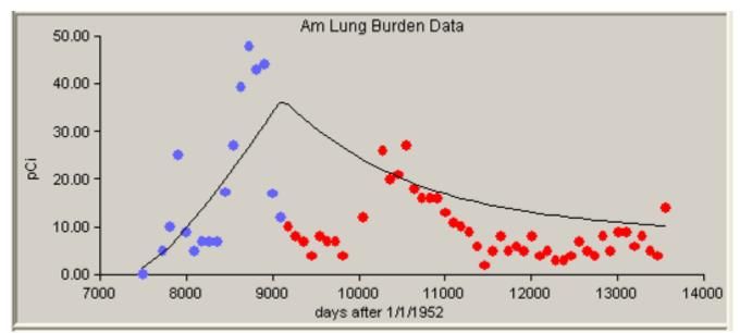
Figure D-43. Predicted americium bioassay results (line) calculated using IMBA-derived americium intake rates compared with measured americium lung burden results (dots), 1/1/1972 to 12/31/1976, 50th-percentile, Type S.
