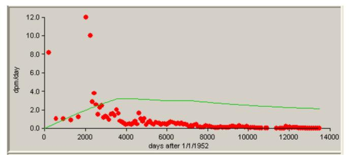
Figure D-42. Predicted plutonium bioassay results (line) calculated using IMBA-derived plutonium intake rates compared with measured plutonium-in-urine results (dots), 1/1/1952 to 12/31/2005, 84th-percentile, Type S.
