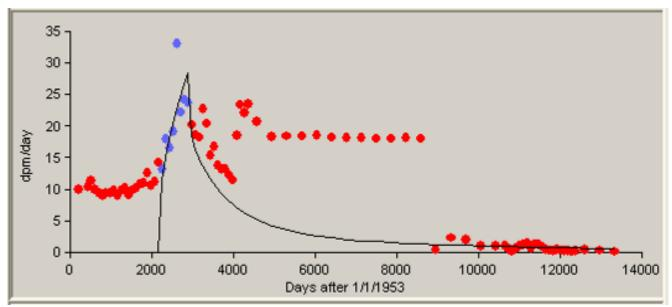
Figure D-15. Predicted uranium bioassay results (line) calculated using IMBA-derived uranium intake rates compared with measured uranium-in-urine results (dots), 1/1/1959 to 12/31/1960, 84th-percentile, Type S.
