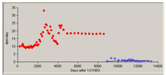
Figure D-18. Predicted uranium bioassay results (line) calculated using IMBA-derived uranium intake rates compared with measured uranium-in-urine results (dots), 1/1/1977 to 12/31/1988, 84th-percentile, Type S.
