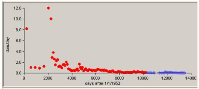
Figure D-28. Predicted plutonium bioassay results (line) calculated using IMBA-derived plutonium intake rates compared with measured plutonium-in-urine results (dots), 1/1/1980 to 12/31/1988, 84th-percentile, Type M.
