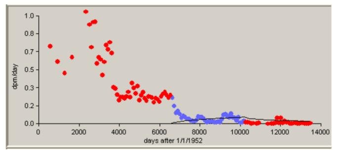
Figure D-23. Predicted plutonium bioassay results (line) calculated using IMBA-derived plutonium intake rates compared with measured plutonium-in-urine results (dots), 1/1/1970 to 12/31/1979, 50th-percentile, Type M.
