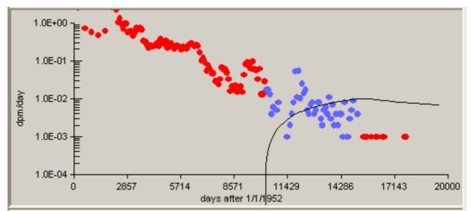
Figure D-34. Predicted plutonium bioassay results (line) calculated using IMBA-derived plutonium intake rates compared with measured plutonium-in-urine results (dots), 1/1/1980 to 12/31/1993, 50th-percentile, Type S.
