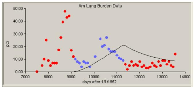
Figure D-44. Predicted americium bioassay results (line) calculated using IMBA-derived americium intake rates compared with measured americium lung burden results (dots), 1/1/1977 to 12/31/1982, 50th-percentile, Type S.
