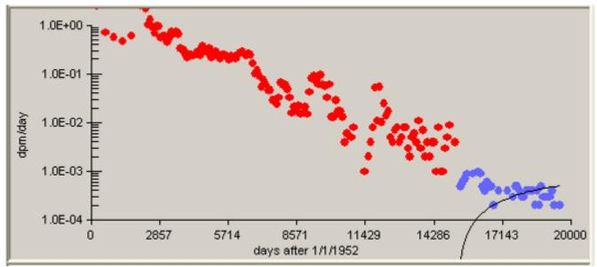
Figure D-35. Predicted plutonium bioassay results (line) calculated using IMBA-derived plutonium intake rates compared with measured plutonium-in-urine results (dots), 1/1/1994 to 12/31/2005, 50th-percentile, Type S.
