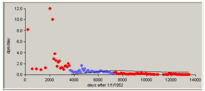
Figure D-37. Predicted plutonium bioassay results (line) calculated using IMBA-derived plutonium intake rates compared with measured plutonium-in-urine results (dots), 1/1/1962 to 12/31/1971, 84th-percentile, Type S.
