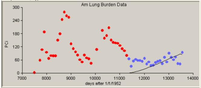
Figure D-48. Predicted americium bioassay results (line) calculated using IMBA-derived americium intake rates compared with measured americium lung burden results (dots), 1/1/1983 to 12/31/1988, 84th-percentile, Type S.
