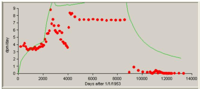
Figure D-19. Predicted uranium bioassay results (line) calculated using IMBA-derived uranium intake rates compared with measured uranium-in-urine results (dots) from all intakes 1/1/1953 to 12/31/1988, 50th-percentile, Type S.
