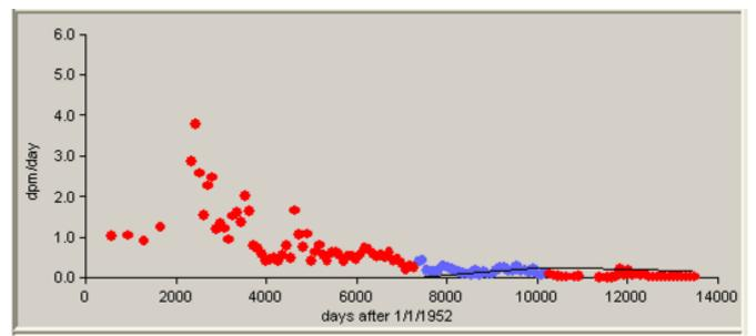
Figure D-38. Predicted plutonium bioassay results (line) calculated using IMBA-derived plutonium intake rates compared with measured plutonium-in-urine results (dots), 1/1/1972 to 12/31/1979, 84th-percentile, Type S.
