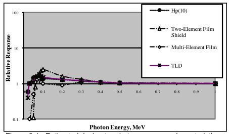
Figure 6-1. Estimated dosimeter photon response characteristics.
