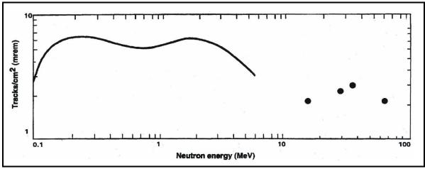
Figure 6-9. Neutron energy response of NTS TED (REECo 1995b).
