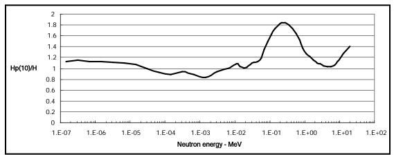
Figure 6-6. Ratio of fluence to dose conversion coefficients for personal dose equivalent  $H_0(10, 0^\circ)$  to conversion coefficients for dose equivalent H.
