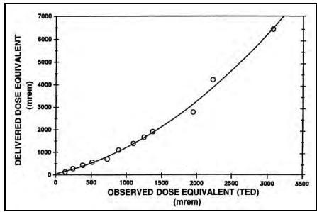
Figure 6-10. Electrochemically etched CR-39 dose response (REECo 1995b).
