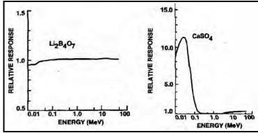
Figure 6-4. Typical photon energy response curves for Li<sub>2</sub>B<sub>4</sub>O<sub>7</sub> and CaSO<sub>4</sub> TLD elements (REECo 1995b).
