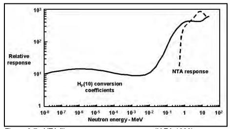
Figure 6-7. NTA film neutron energy response (IAEA 1990).
