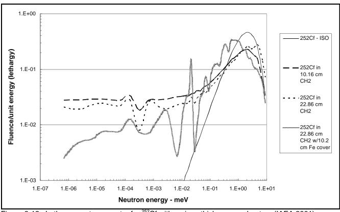
Figure 6-12. Lethargy neutron spectra for <sup>252</sup>Cf with various thickness moderators (IAEA 2001).
