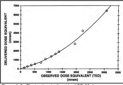
Figure A-6. Electrochemically etched CR-39 dose response (Allen and Schoengold 1995).
