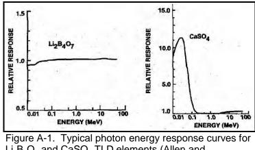
$Li_2B_4O_7$  and  $CaSO_4$  TLD elements (Allen and Schoengold 1995).
