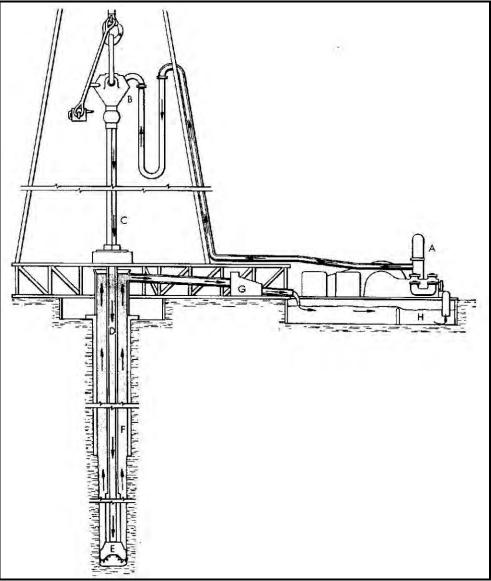
Figure D-5. Circulation of drilling fluid.
