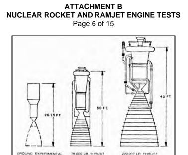
Figure B-5. Nuclear rocket engine configurations (NASA 1991).
