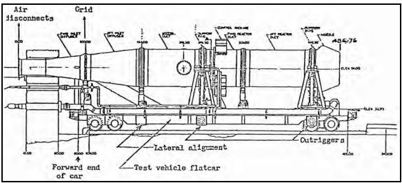
Figure B-6. Schematic diagram of TORY II-C reactor on vehicle flatcar.
