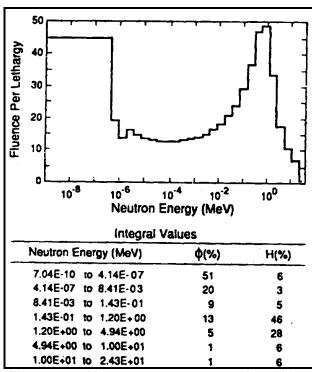
Figure 6-7. Neutron spectrum near door K in SNM Vault at Plutonium Facility (Harvey and Hainal 1993).
