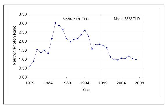
Figure 6-3. Geometric mean of neutron-to-photon ratios for records with both deep dose and neutron dose of 50 mrem or greater, 1979 to 2004 (LANL 2004, updated January 2009).
