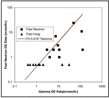
Figure 6-17. Correlation of fast neutron dose equivalent to gamma dose at MTR.
