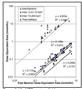
Figure 6-16. MTR neutron field components.
