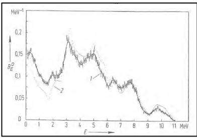
Figure 6-8. Probability density of neutron spectrum from a  $^{241}$ Am-Be ( $\alpha$ ,n) source (Kluge and Weiss 1982).
