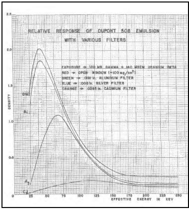
Figure 6-7. Response of DuPont 508 film with various filters to 140 mrem uranium beta and 100 mR of different energy photon irradiation. The original badge used the open window and cadmium shielded films. The multiple filter badge used all three filters plus the open window (Cipperley and Gammill 1959).
