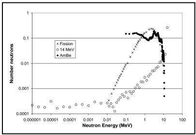
Figure 6-14. Neutron spectra simulating INEEL facilities.
