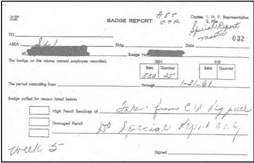
Figure 6-5. Special badge report associated with a high beta reading listed in Figure 6-4.
