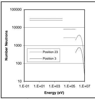
Figure 6-15. Sample MTR spectra from Hankins Bonner measurements.
