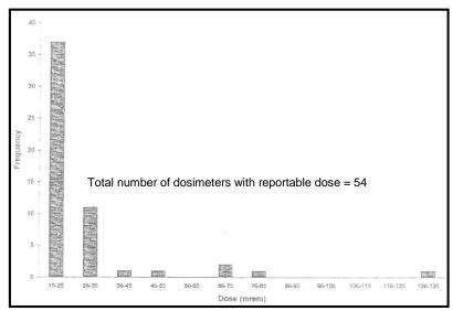
Figure 6-12. Distribution of reportable neutron dose for the first 9 months of 1995. Of 1,461 dosimeters, 1,407 were below the 15 mrem reporting level.
