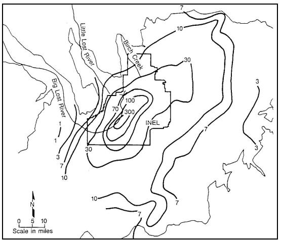
Figure 4-3. Nine-year (1974 - 1983) average mesoscale dispersion isopleths of air concentration at ground level ( $hr^2/m^3 \times 10^{-9}$ ), normalized to unit release rate (Bowman 1984).
