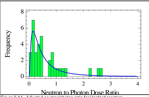
Figure 6-14. Adjusted neutron/photon ratio for Hanford reactors.
