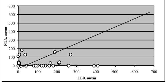
Figure 6-7. Comparison of Hanford PFP workplace NTA and HMPD neutron dose (Nichols et al 1972).
