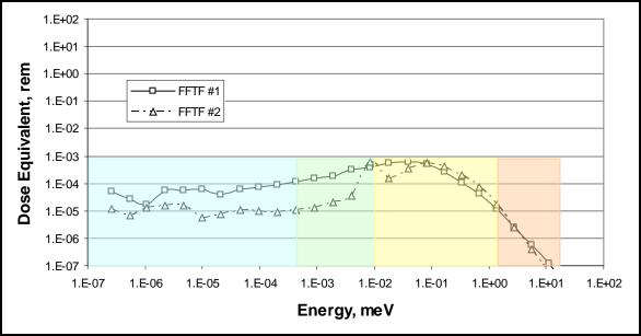
Figure 6-9. Neutron spectra for Hanford 400 Area FFTF.
