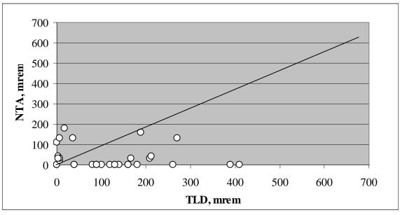
Figure 6.3.4.4-1. Comparison of Hanford PFP workplace NTA and HMPD neutron dose. (Nichols et al 1972)
