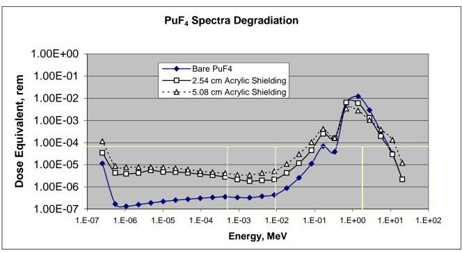
Figure 6.3.4.5-1. Degradation in neutron energy spectra for bare, 2.54 cm and 5.08 cm of acrylic plastic shielding with neutron energy groups overlay.
