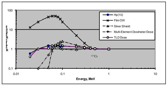
Figure 6.3.3.1-1. Measured Hanford dosimeter photon response characteristics. (Wilson et al 1990)
