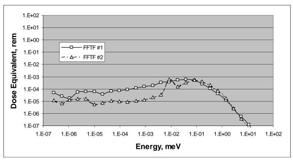
Figure 6.3.4.5-4. Neutron spectra for Hanford 400 Area FFTF.
