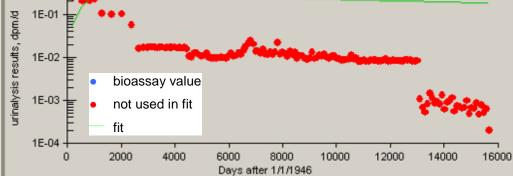
Figure C-16. Predicted 50th-percentile urinary excretion of Type S plutonium from 1946 to 1988 based on four independent intakes, compared to bioassay data.
