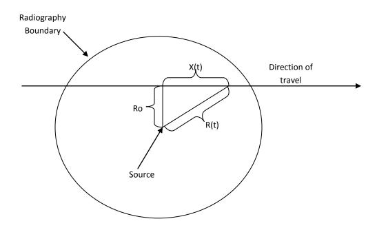
The dose received by an individual walking through a radiography area can be calculated using the diagram provided above. The source is represented by the center of the circle while the circle represents the delineated boundary of the radiography area. The horizontal arrow represents the path taken by the individual through the delineated area. The closest distance the person come to the source is indicated as Ro and the distance from the source at any time t is R(t).
