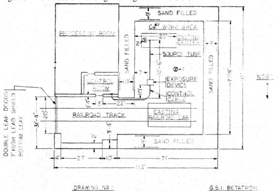
DRAWING Nº ! 80 CURIE SOURCE G.S.I. BETATRON CONCRETE BLOCK WALLS, MCRIAR FILLED, 25'HIGH
