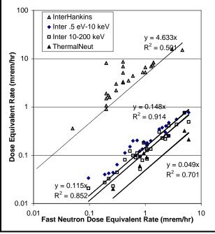
Figure 6-15. MTR neutron field components.
