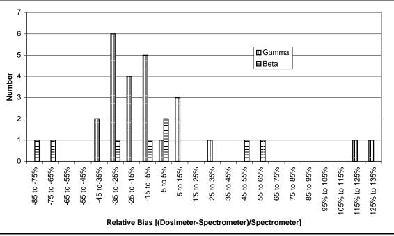
Figure 6-9. Gamma and beta radiation field characterization.
