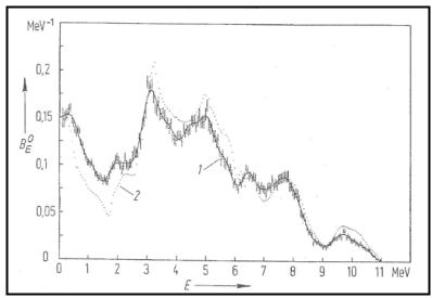
Figure 6-8. Probability density of neutron spectrum from a  $^{241}$ AmBe ( $\alpha$ ,n) source (Kluge and Weise 1982).
