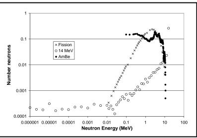
Figure 6-13. Neutron spectra simulating INEEL facilities.
