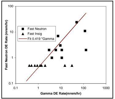
Figure 6-16. Correlation of fast neutron dose equivalent to gamma dose at MTR.
