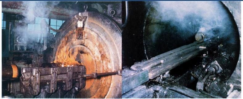
Billet being forced into extrusion die; flames are lubricant ignited by the hot die.
