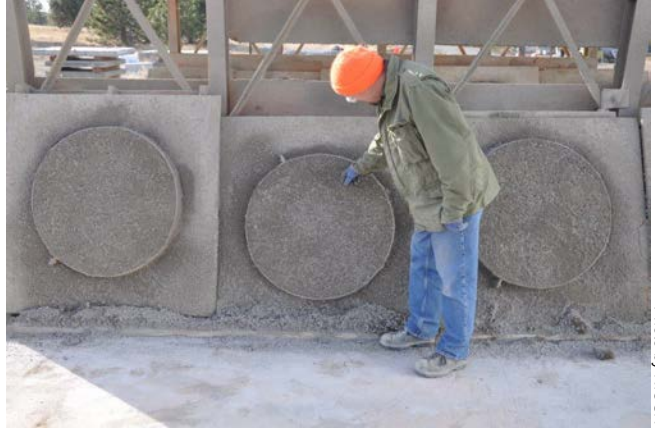
Figure 76. Sprayed round-panel shotcrete samples.
