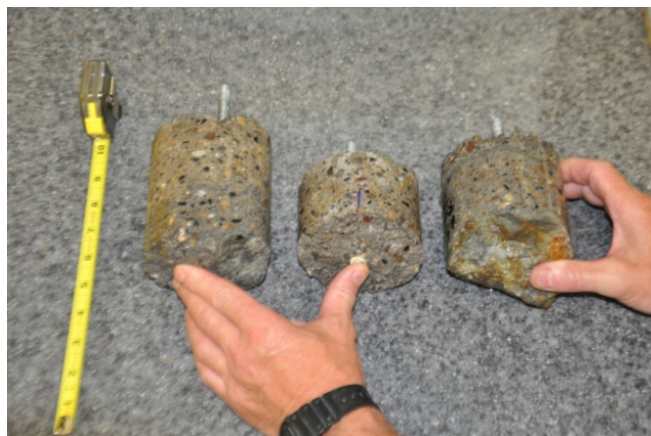
Figure 71. Adhesion test cores showing two breaks in shotcrete (left, test 1 and middle, test 2), and one break in host rock (right, test 3).
