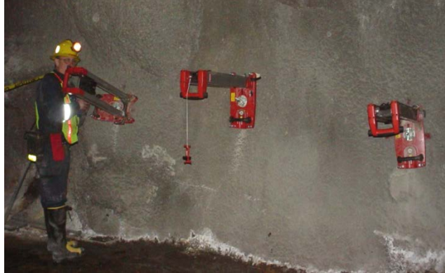
Figure 62. Shotcrete adhesion test site with three drill stands mounted on mine rib.
