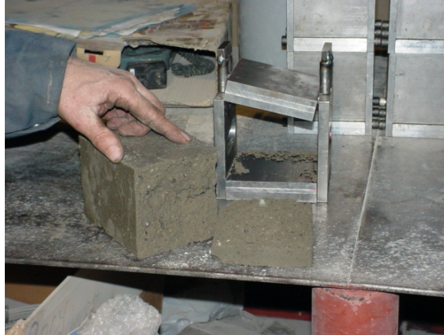
Figure 50. Shotcrete sample showing exposed failure plane.
