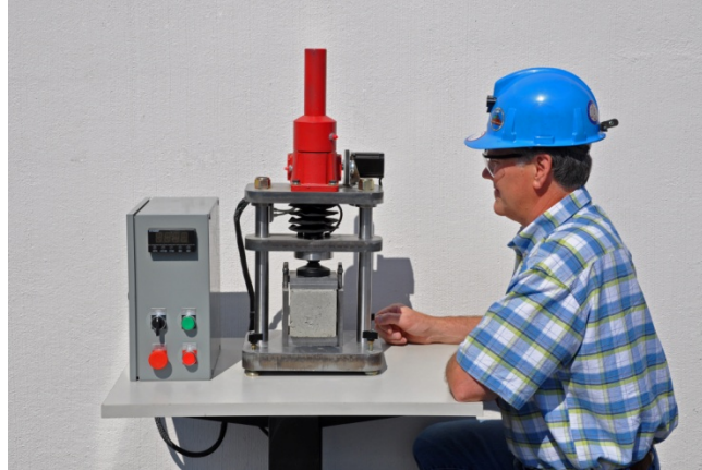
Figure 35. Operation of portable shotcrete test machine.
