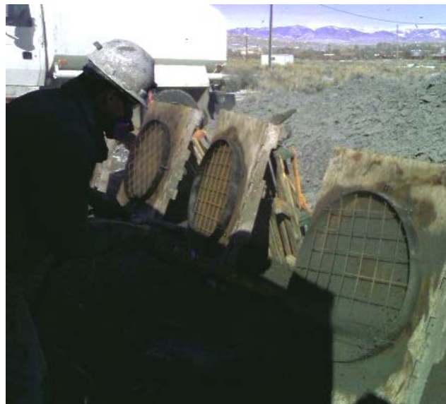
Figure 86. Spraying round-panel shotcrete samples reinforced with wire mesh.
