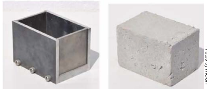
Figure 37. Partial-beam shotcrete mold (left) and shotcrete test sample (right).
