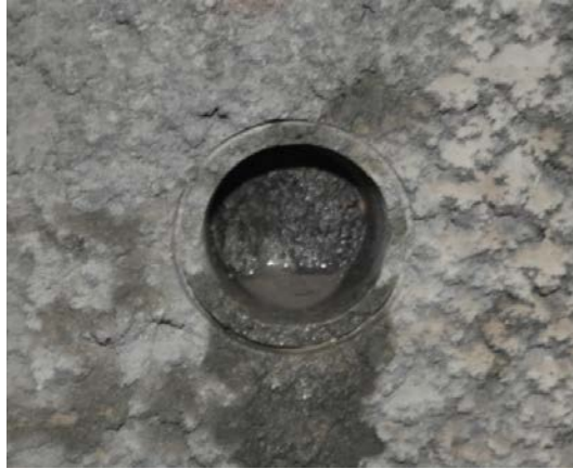
Figure 66. Adhesion test #1: core broke in shotcrete and at interface between two shotcrete layers.
