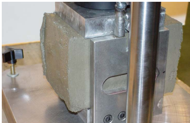
Figure 39. Loading of a partial-beam shotcrete sample during an early strength test.
