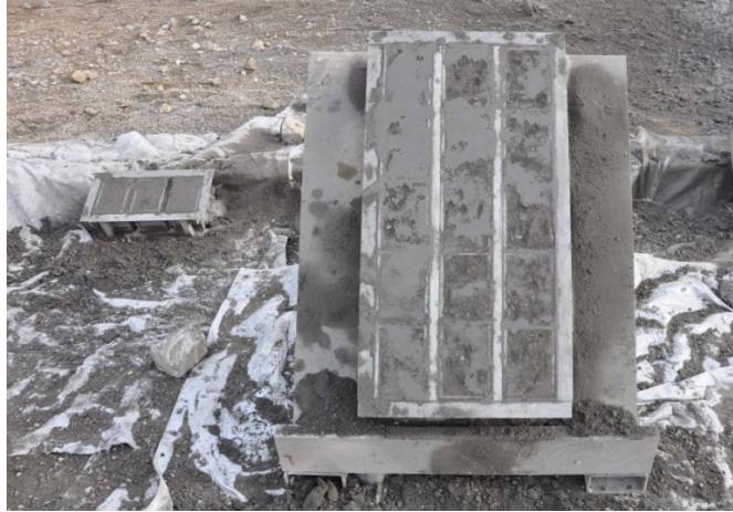
Figure 38. Containment fixtures and molds for making partial-beam shotcrete samples (large, center; small, upper left).
