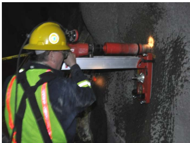
Figure 64. Wet drilling a 102-mm (4-in) diameter hole for the shotcrete adhesion test core (note bit change).
