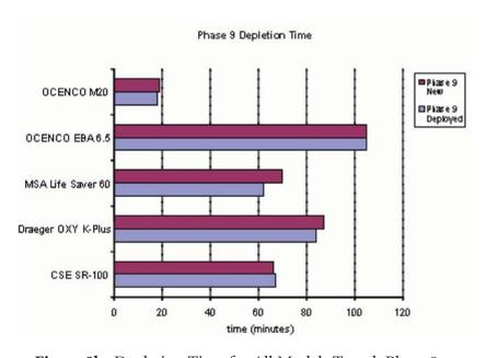
Figure 8b. Depletion Time for All Models Tested–Phase 9
