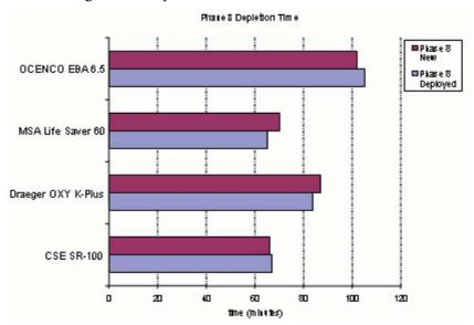
Figure 8. Depletion Time for All Models Tested
