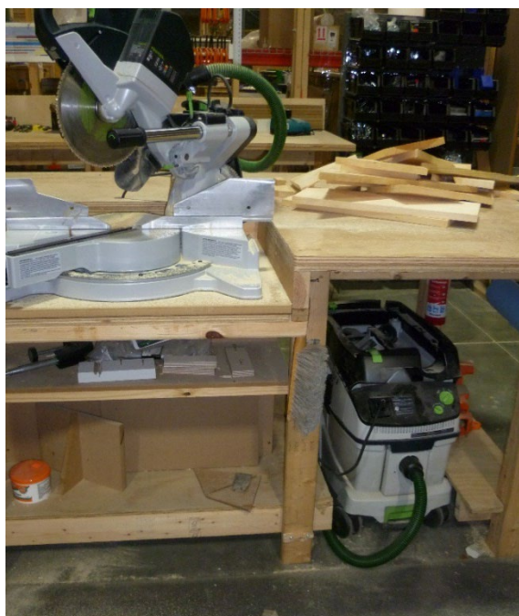
Figure B2. Compound miter saw connected to a mobile dust extractor. Photo by NIOSH.
