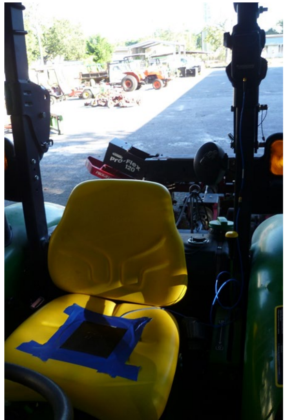
Figure B1. Rubber seat pad with embedded triaxial sensor for measuring whole-body vibration on the groundskeeping tractor seat. Photo by NIOSH.
