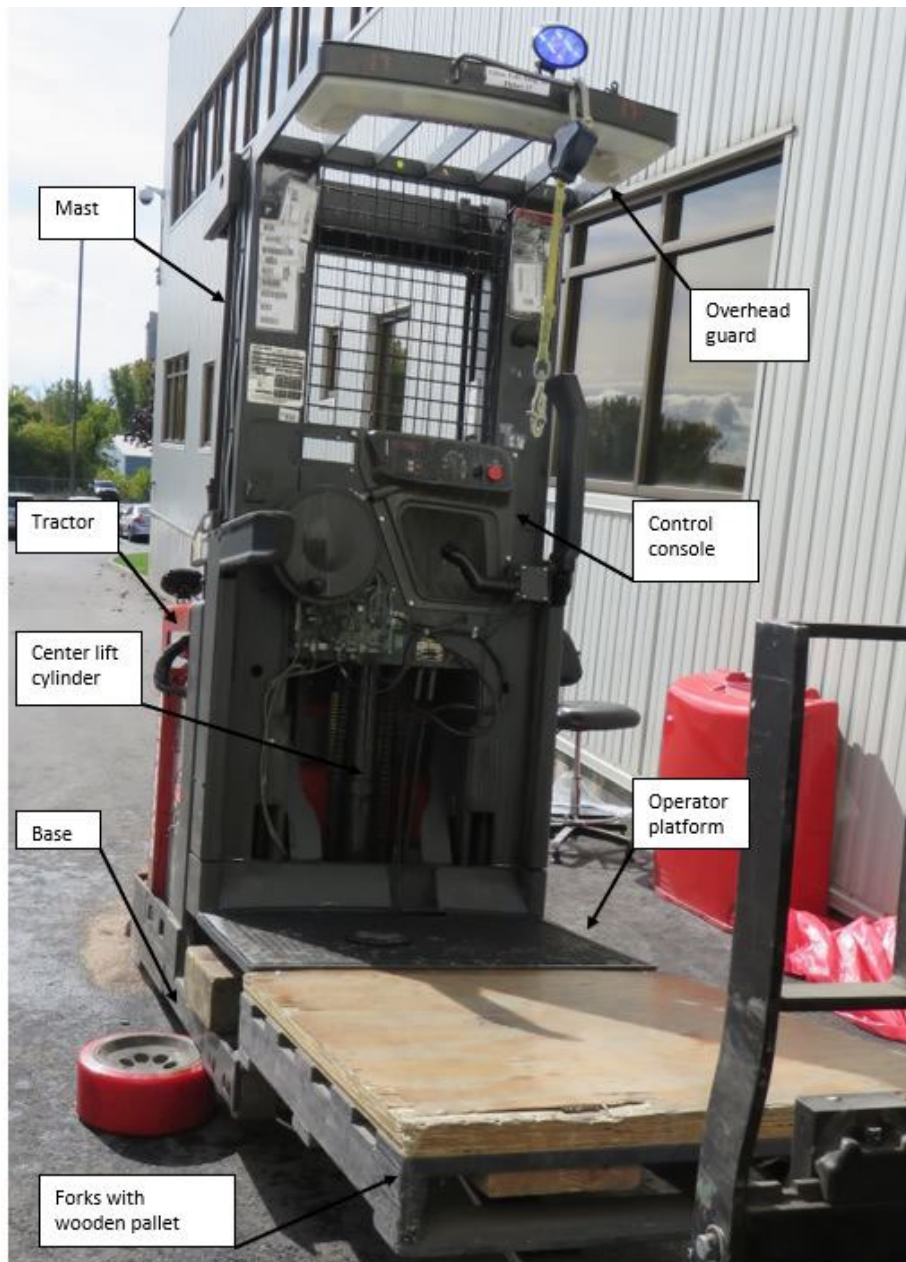
Photo 1. The order picker that was involved in the incident with the console cover removed (Photo courtesy of OSHA).
