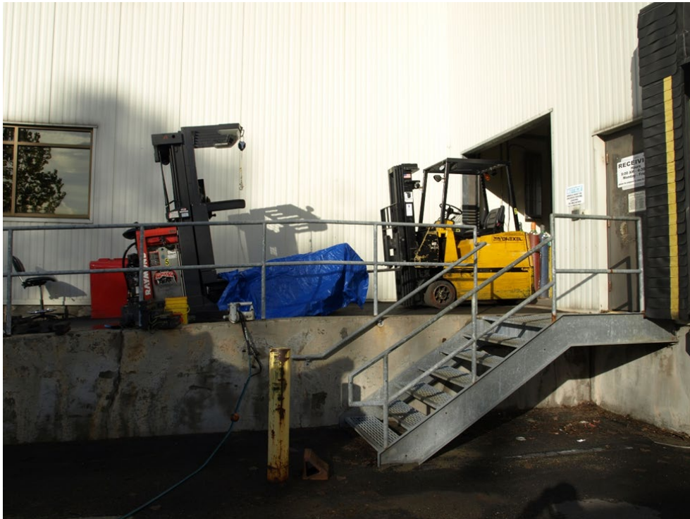
Photo 2. Post incident scene: The order picker was parked on the inclined ramp outside the loading dock during the incident. The forklift on the right was used in the rescue to lift the platform off the victim (Photo courtesy of city police department).
