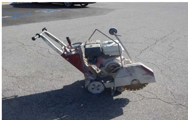
Exhibit 1: The gasoline-powered concrete saw used by the victim.
