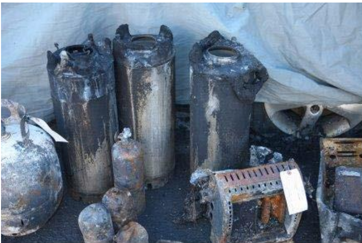
Photo 3: Incident propane cylinders and space heater.
