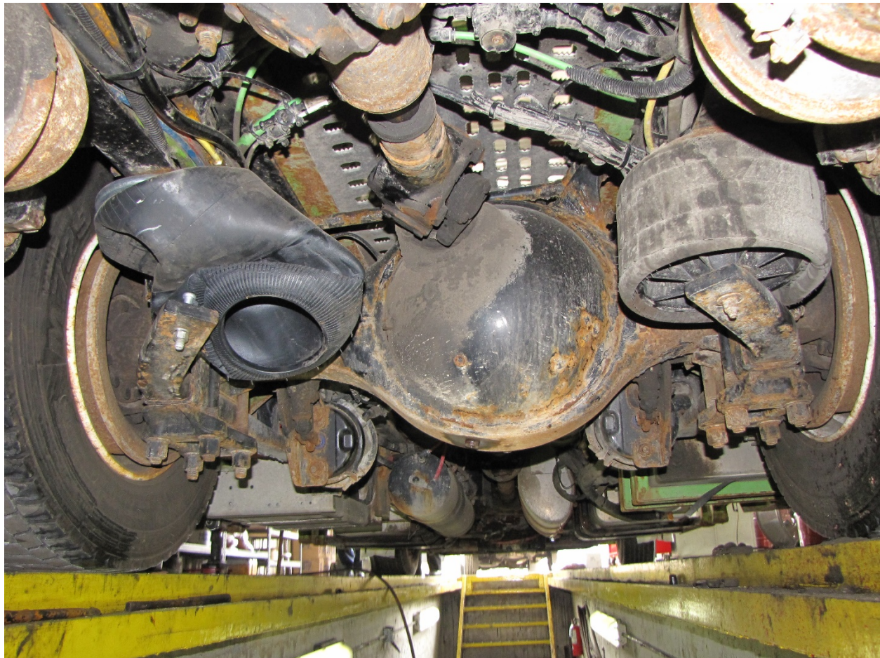
Figure 6. Air spring after the explosion.
