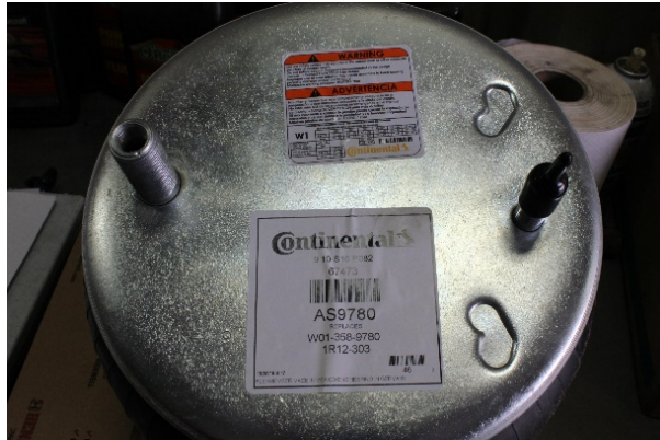
Figure 2. Sample of a new air suspension air bag to be installed.
