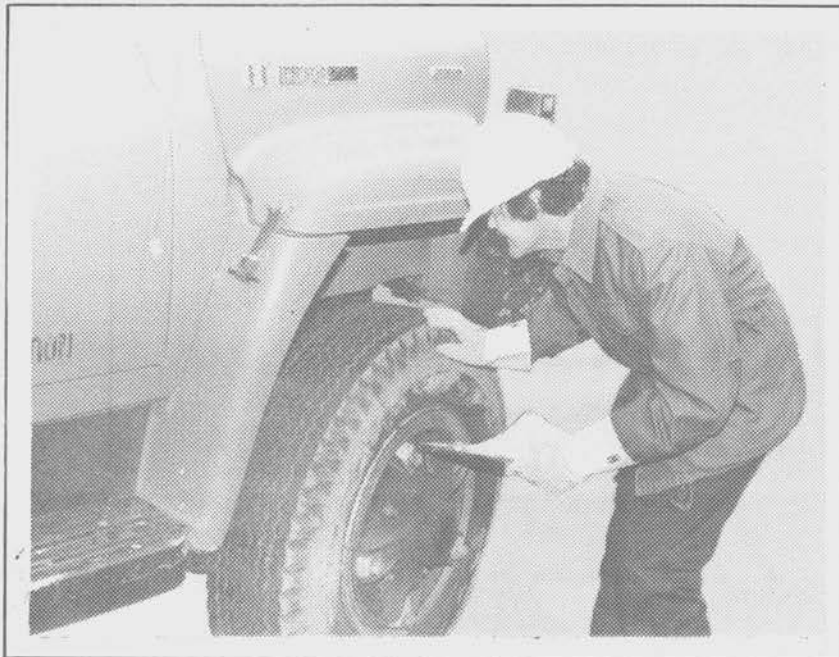
Figure 2. Checking tires for cuts, gouges, underinflation.
