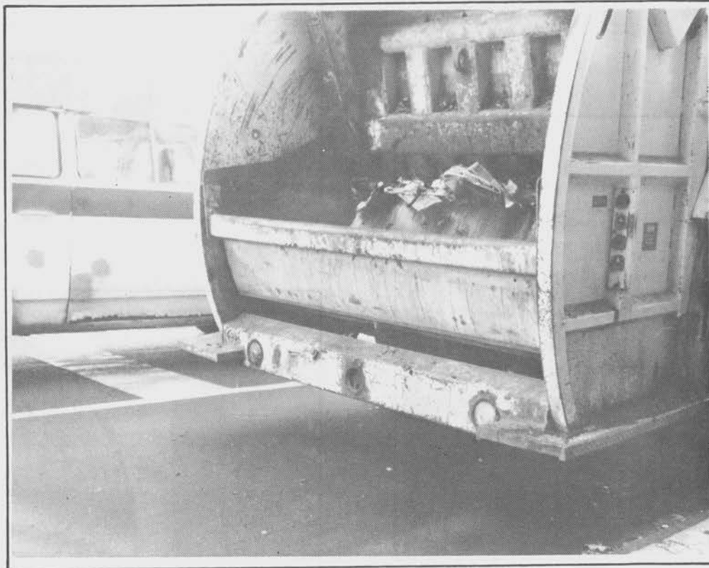
Figure 88. Control panel is too low if children can reach it.
