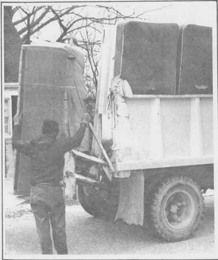
Figure 47. Keep clear of shear point (lift arms) as gate is raised.
