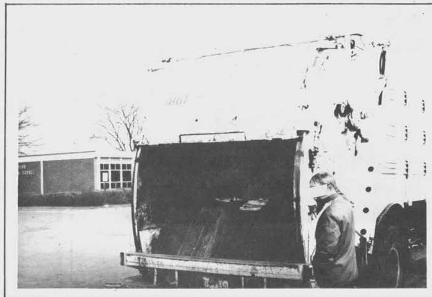
Figure 81. Rolling guard door. open.
