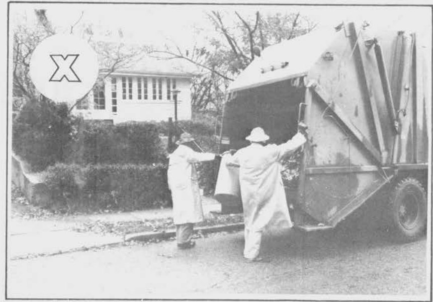
Figure 73. Operating packer with right hand, dumping load with left.
