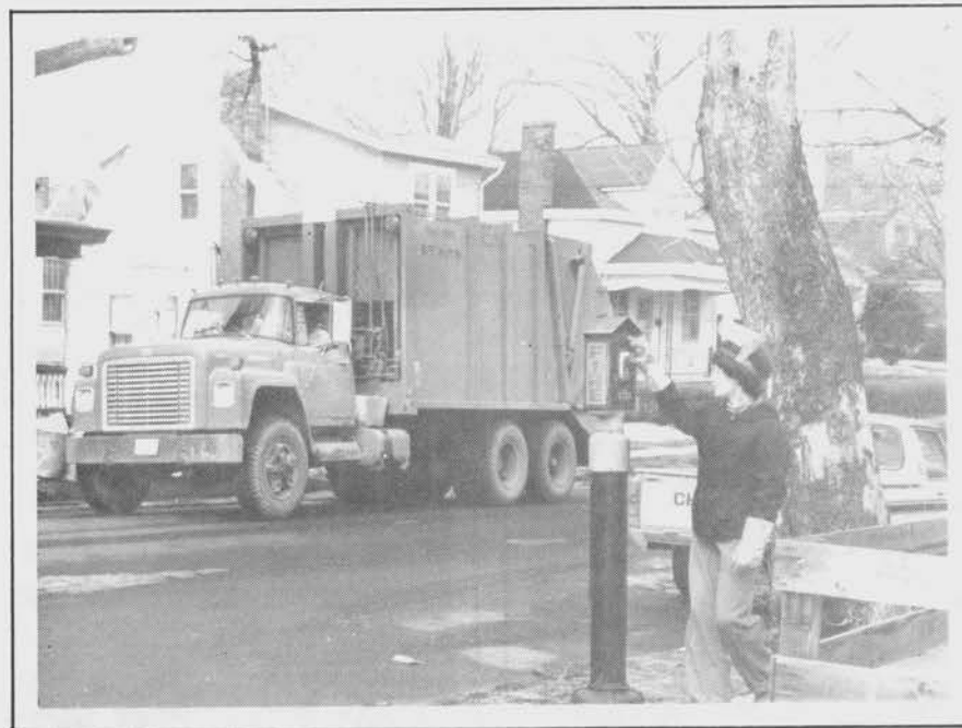
Figure 111. Calling fire department to report hot load or truck fire.
