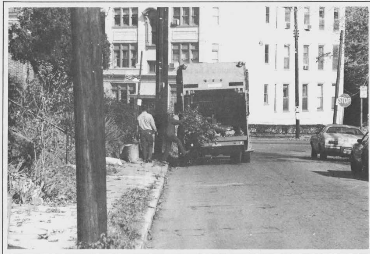
Figure 34. When truck is on left side of street, packer controls are on the traffic side.
