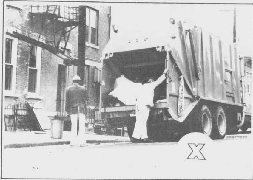
Figure 72. Operating packer with right hand, positioning oversized refuse with left.
