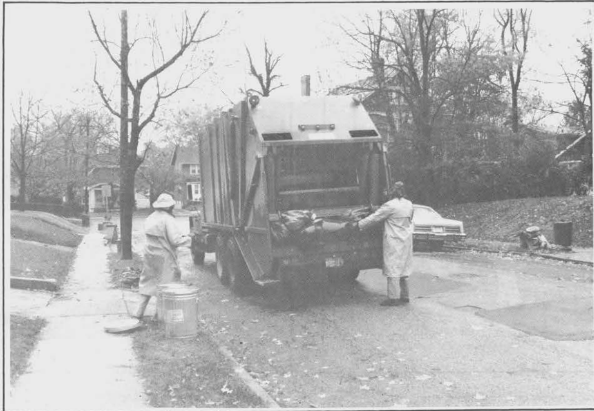
Figure 71. Operating packer with right hand, pushing bulging bags with left.
