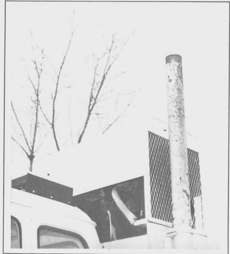
Figure 104. Vertical exhaust outlet (preferred).
