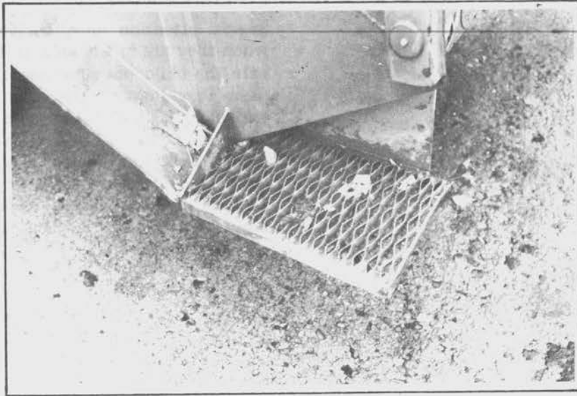
Figure 56. Self-cleaning riding step.
