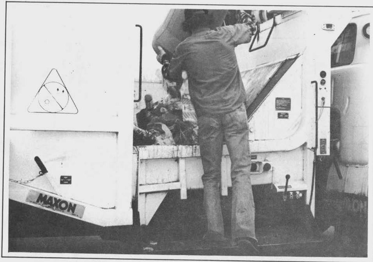
Figure 38. Lifting from the step level.
