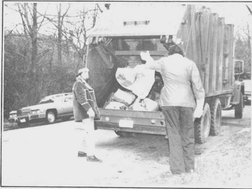
Figure 55. This bag is about to bounce out of the hopper and burst.
