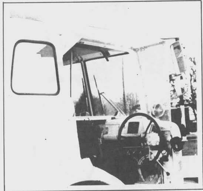
Figure 14. Rain canopy on side-driving controls.
