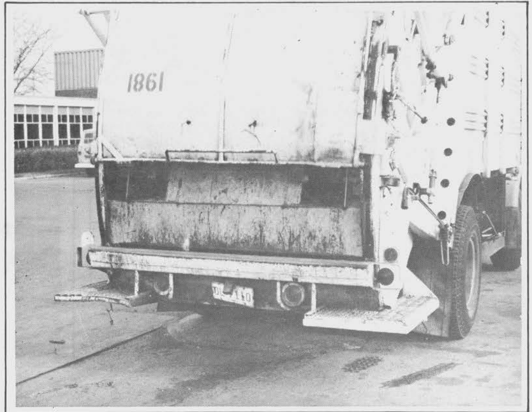
Figure 83. Guard door reopens after packer panel clears loading sill.
