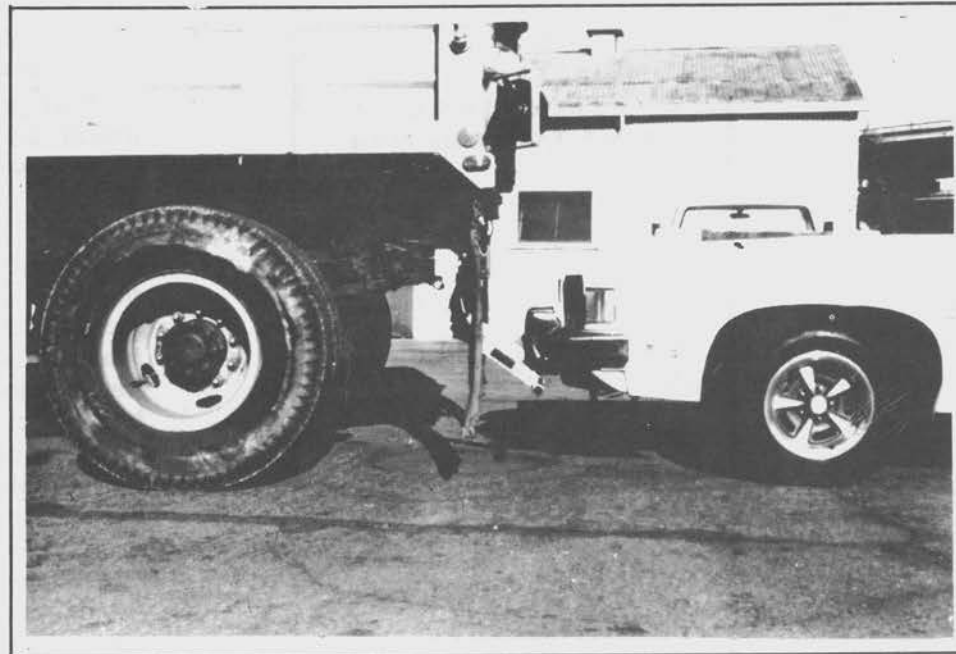
Figure 17. Pressure-sensitive backup safety device.
