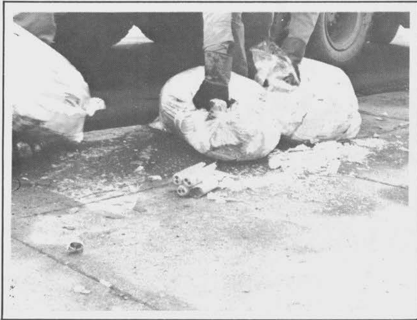
Figure 105. Tubes here fell out of the can when the can was carried.
