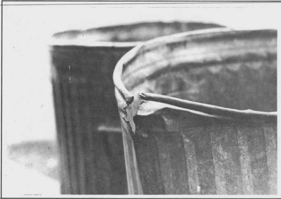
Figure 20. Tag a can with a jagged edge as unacceptable.
