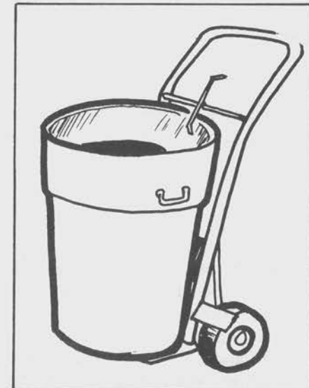
Figure 33. Use hand truck to get tub up or down stairs or slopes, or for tubs lacking wheels.
