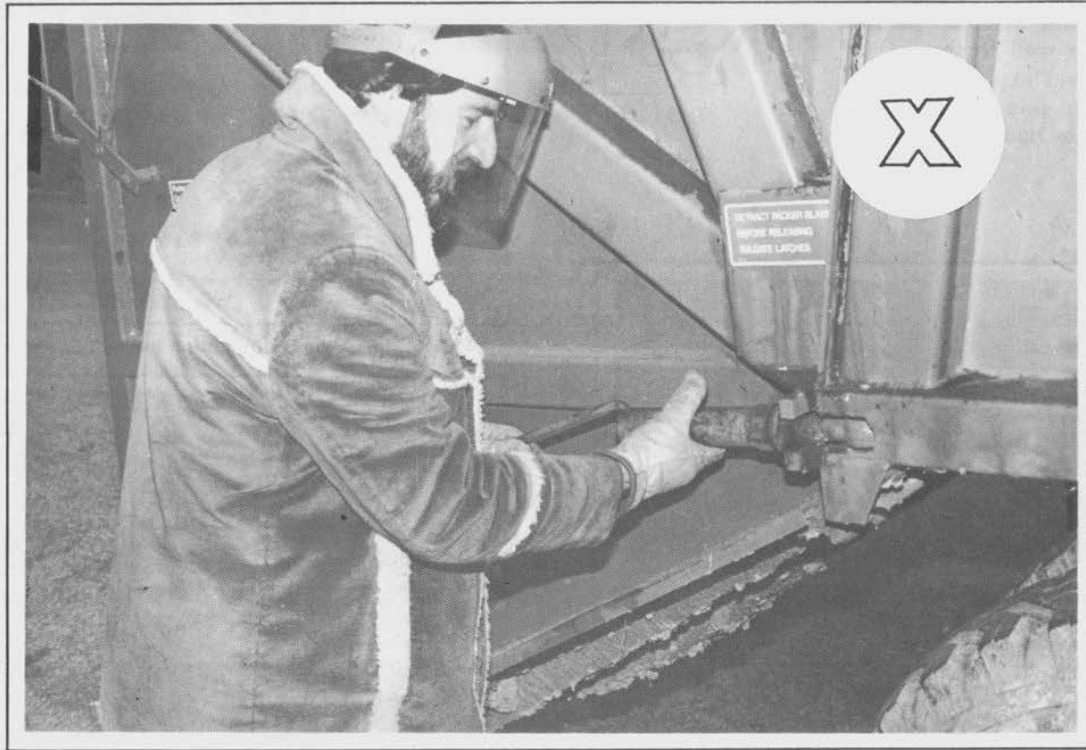
Figure 108. Loosening turnbuckle to overload can have deadly results.
