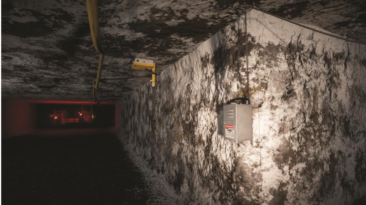
Figure 11. Screenshot of mesh node and mine phone digital assets in VR Mine. These assets can be used to play a pre-recorded message or send a communication during a training scenario. VR Mine provides context to the message content through the dynamic events of a staged scenario.
