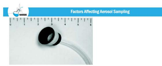
Figure 2F. Bell mouth cowl sampler. An alternative to the standard asbestos sampling cassette. The inlet is flared to reduce the effect of external air motion on sample uniformity. It is made of conductive plastic and is operated at a flow rate between 0.5 L/min to 16 L/min.
