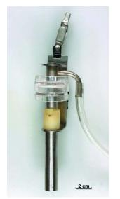
Figure 2G. Dorr-Oliver 10-mm nylon cyclone. It is used as a respirable sampler most often at 1.7 L/min. A version of this sampler is used at 2 L/min in coal mines with a 1.38 correction factor applied to the resultant mass. The holder encases body of the cyclone so that only the inlet section is visible just below the connection to the 37 mm cassette. The coal mine dust sampler version uses a cassette with an aluminum cartridge encasing the collection filter.
