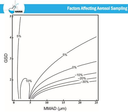
Figure 3. Bias map for the 10-mm nylon cyclone (operated at 1.7L/min) compared with the respirable convention [Courbon et al. 1988]. The contour lines represent percent bias for specific lognormal size distributions. The calculation of this map is based on laboratory measurement of cyclone penetration and can be used with field size distributions to estimate sampling bias.
