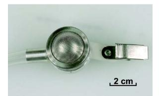
Figure 2D. Button sampler. So-named because the inlet, a hemispherical screen with ~380  $\mu$ m diameter holes, resembles a large button. It was developed as an inhalable sampler with reduced wind direction response and improved filter deposit uniformity. The sampler uses metal construction and operates at 4 L/min.
