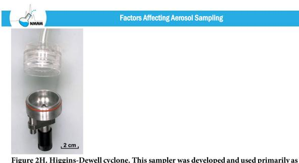
Figure 2H. Higgins-Dewell cyclone. This sampler was developed and used primarily as a respirable sampler in the UK. This version provides an interface directly to a 37-mm cassette. Cyclone construction is steel and operates at 2.2 L/min.
