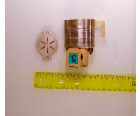
Figure 2J. Personal cascade impactor sampler (model Marple 290, Thermo Fisher Scientific). The sampler has five stages in the version shown and an additional three stages are available to provide cutpoints from 0.4  $\mu$ m to 21  $\mu$ m. The flap over the inlet reduces direct projection of large particles into the inlet. This sampler allows measurement of aerosol size distribution and calculation of respirable and thoracic fractions. It is constructed of aluminum and operates at 1.7 L/min.
