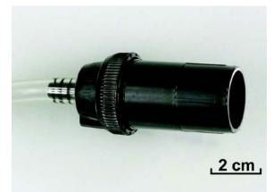
Figure 2E. Asbestos sampling cassette. The long (50 mm) inlet was designed to prevent incidental contact with the filter surface and, when facing downward, acts to a certain extent as an elutriator, preventing larger particles from reaching the filter surface. It is made of conductive plastic and is operated at a flow rate between 0.5 L/min to 16 L/min.
