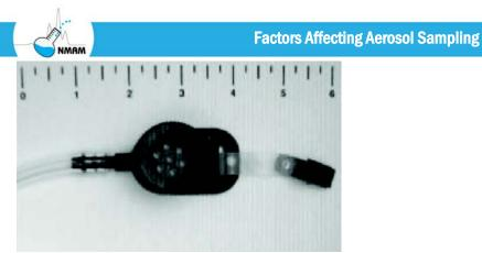
Figure 2C. Seven hole sampler used for inhalable dust sampling in the UK. Sampler is made of conductive plastic and operates at 2 L/min.
