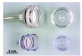
Figure 2A. 37-mm (top) and 25-mm (bottom) filter cassettes. Open faced cassettes are shown on left. Closed-faced cassettes include placement of clear piece (on right) over filter. These are shown in acrylic copolymer (clear, non-conducting) material and are more prone to electrostatic losses. Other construction materials are available, including conducting plastic. Sampling flow rates range from 0.5 to 10 L/min.
