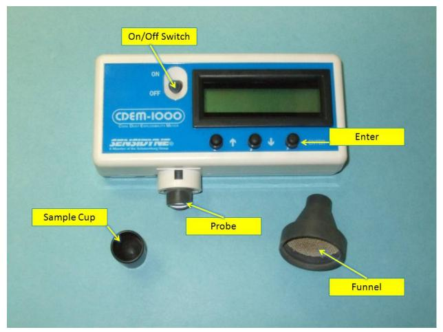
Figure A1. Coal Dust Explosibility Meter (CDEM).
