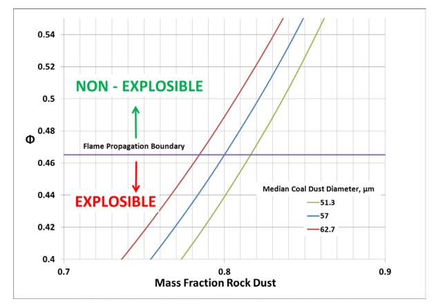
Figure D1. A comparison of coal dust particle size distributions on  $\phi$  values. Rock dust particle size distributions are constant.
