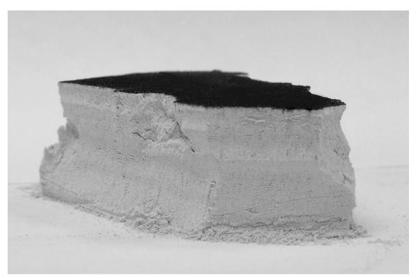
Figure E1. Cross section of a very thin (0.01-in-thick) explosible float coal dust layer deposited on top of a 3/4-in-thick (20-mm-thick) layer of rock dust [NIOSH 2006].
