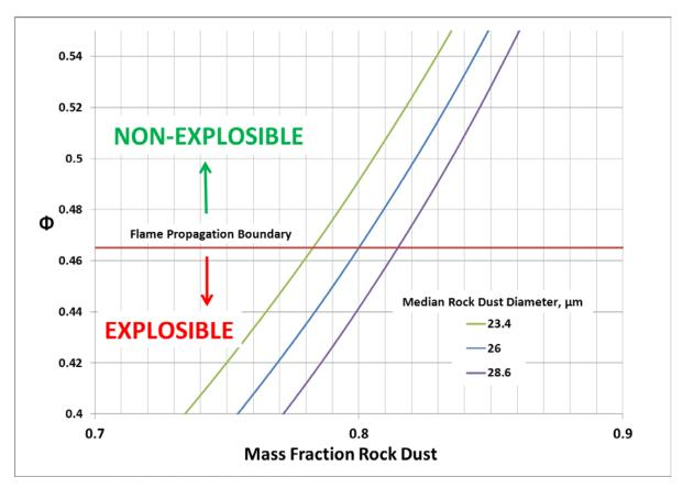
Figure D2. A comparison of rock dust particle size distributions on  $\phi$  values. Coal dust particle size distributions are constant.
