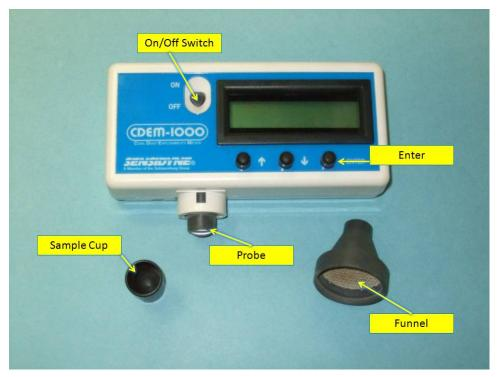
Figure 2. Coal Dust Explosibility Meter (CDEM).
