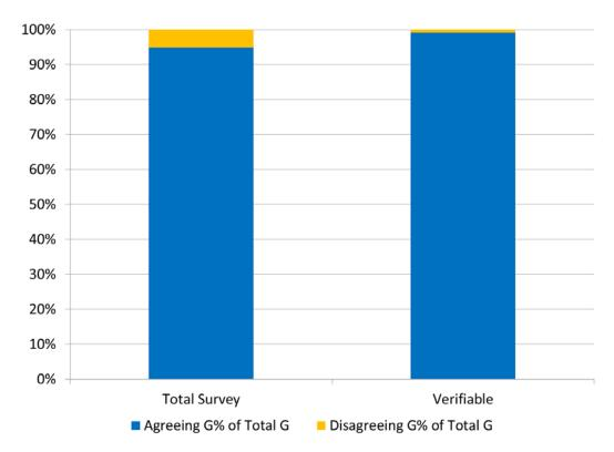
Figure 5. CDEM GREEN (G) measurement comparison of NIOSH-received samples. Agreeing GREEN samples have LTA results > 80% IC. Disagreeing GREEN samples have < 80% IC LTA results.
