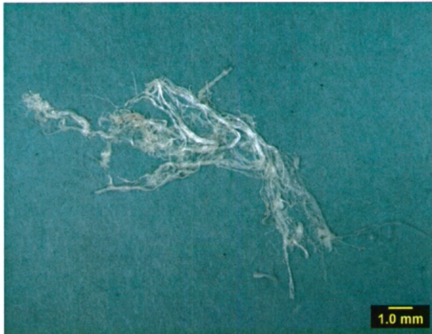
Figure 2a. Optical Image of Chrysotile Grade 4 (insulation/cement pipe grade).
