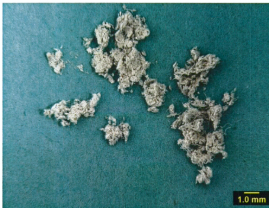
Figure 3a. Optical Image of Chrysotile Grade 7 (friction parts grade).
