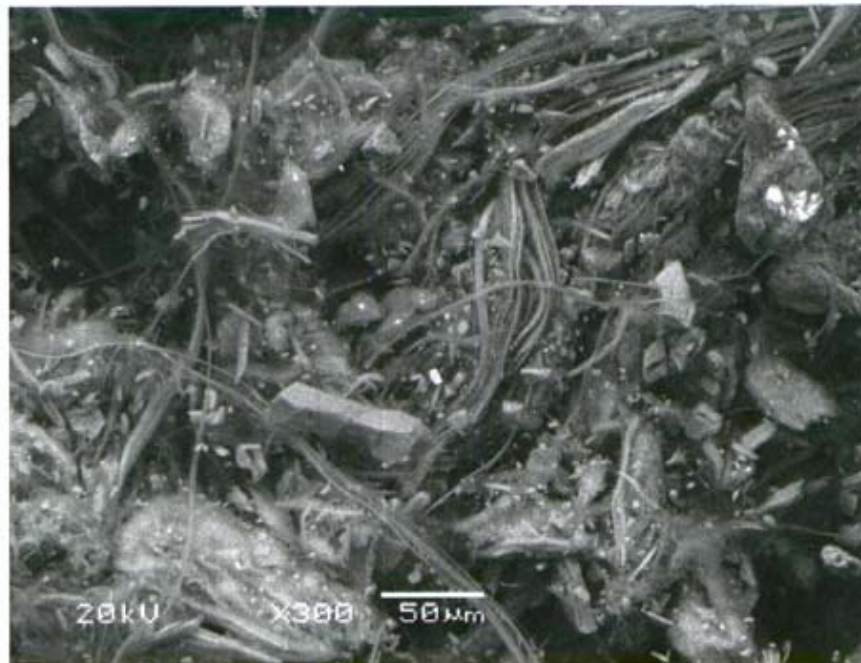
Figure 4b. SEM Image of Chrysotile Ore (Quebec chrysotile miner exposure).
