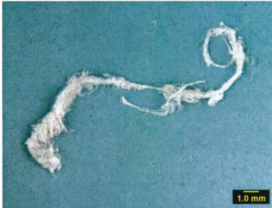
Figure 1a. Optical Image of Chrysotile Grade 3 (textile grade).
