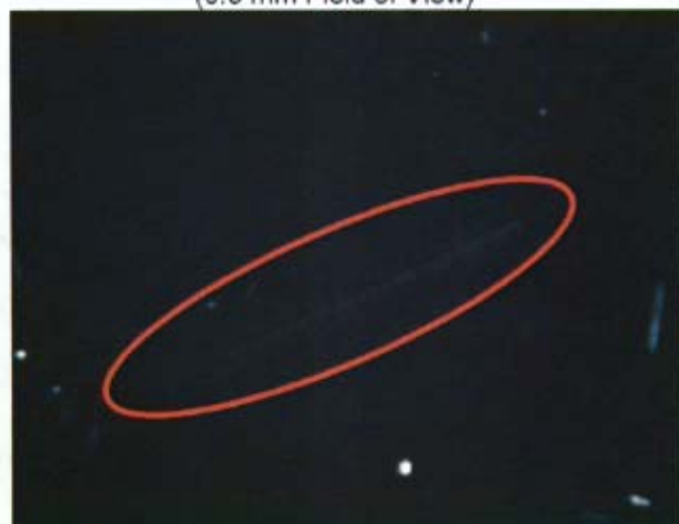
Nonasbestos: oblique extinction (0.5 mm Field of View)
