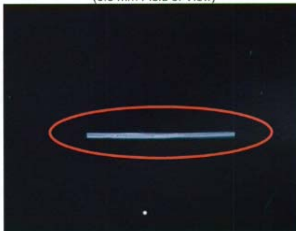
Nonasbestos: visible in parallel orientation (0.5 mm Field of View)
