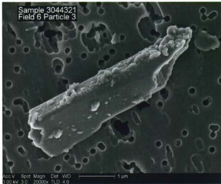
Figure 21. SEM Micrograph of an amphibole crystal from an El Dorado Hills soil sample
