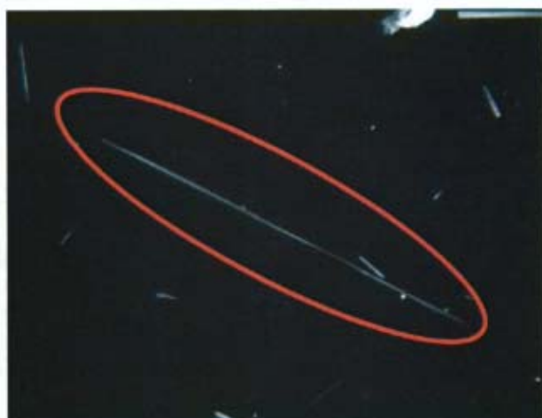
Asbestos fiber: visible at an oblique angle (0.5 mm Field of View)
