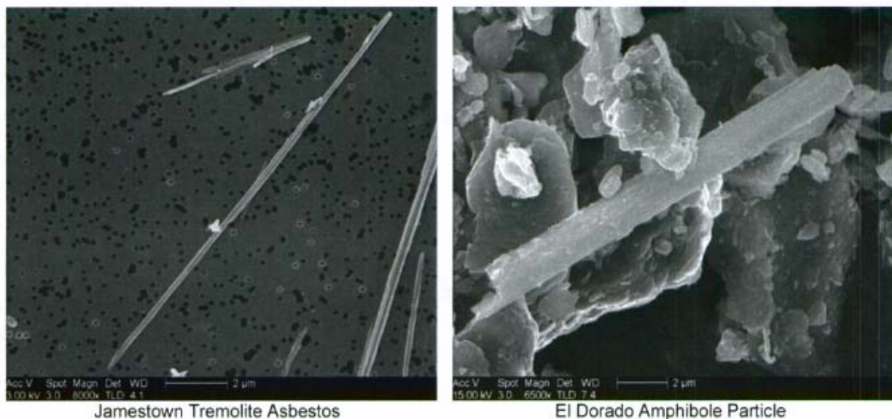
Figure 16. Comparison of the morphology of particles observed in the Jamestown tremolite asbestos sample with that of amphibole particles observed in the El Dorado Hills soil samples.
