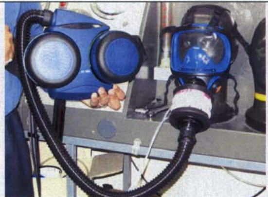
SR500 with flow meter in hose
