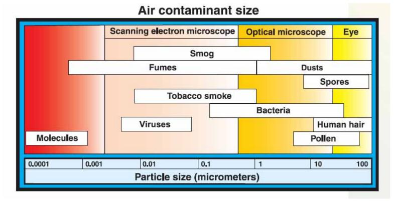
Adapted from: Guidance for Filtration and Air-Cleaning Systems to Protect Building Environments from Airborne Chemical, Biological, or Radiological Attacks, DHHS (NIOSH) Publication No. 2003-136.
